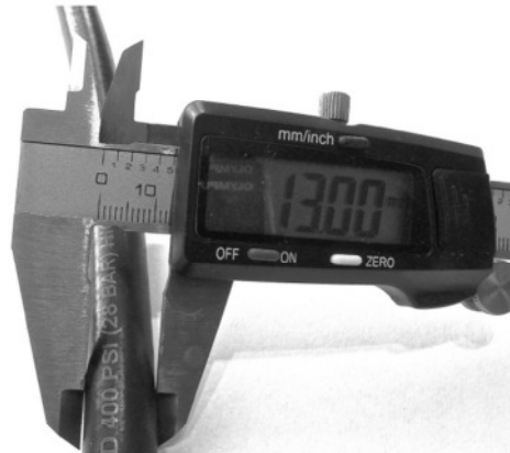
New standard type 13 mm diameter MP hose
