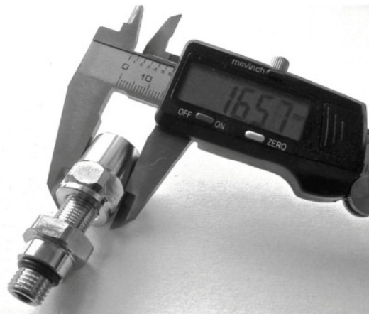
New type hose end (EV50 hose): 16.5 mm diameter
