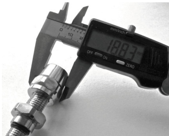
Old type hose end (AP150 hose): 18.8 mm diameter
