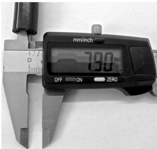
Old Auto Air-only 14 mm diameter MP hose
