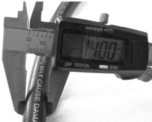
Old Auto Air-only 14 mm diameter MP hose
